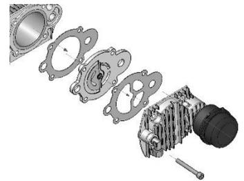
**REPLACING THE 2<sup>ND</sup> STAGE VALVE:**
