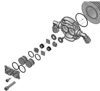
**REPLACING THE 3<sup>RD</sup> TO 4<sup>TH</sup> STAGE VALVE:**
