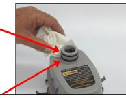
Apply a light coat of Silicone grease to O-Rings. Do not use automotive or Marine Grease!
