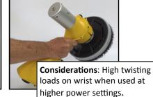
One-handed, grip around the motor housing, right hand...
