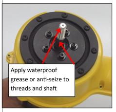
Clean & lubricate drive shaft, drive hub & Spinner Nut
