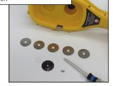
Stack the desired 1-1/2" ¼"hole stainless fender washers in the compartment.
