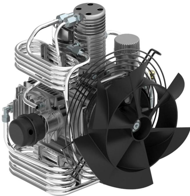
The crankshaft bearings are all made in Europe and their high quality guarantees the compressor a longer lifetime. Cooling of the compressed air is done through the inter-stage aluminum and stainless steel cooling coils system. This is a small-sized compressor with 4 compression stages with all piston rings made in cast iron providing high performance over the time.
