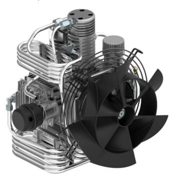
The crankshaft bearings are all made in Europe and their high quality guarantees the compressor a longer lifetime. Cooling of the compressed air is done through the interstage aluminum and stainless steel cooling coils system. This is a small-sized compressor with 4 compression stages with all piston rings made in cast iron providing high performance over the time.
